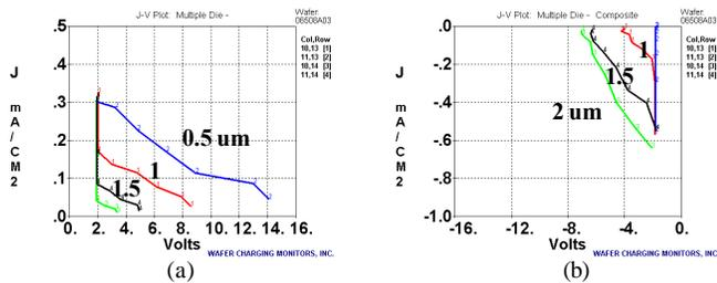
Figure 9. J-V plots for 2µm, 1.5µm, 1µm, and 0.5µm holes obtained in a non-uniform plasma oxide etcher. (a) positive J-V, (b) negative J-V.
