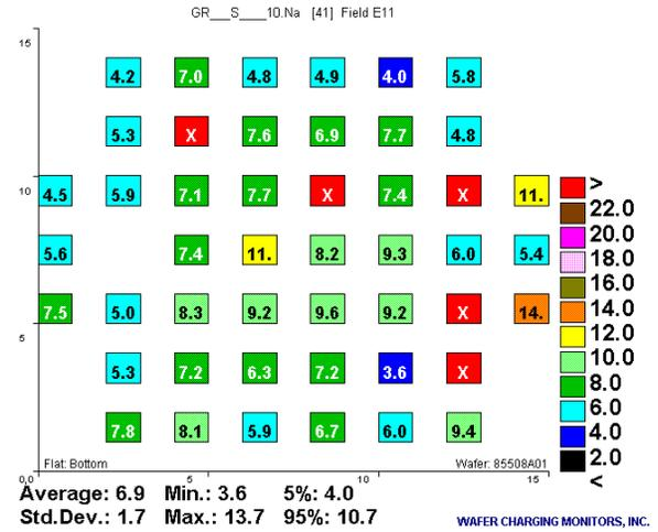
Figure 7. Positive voltage response seen after exposure to Ar plasma with RF bias
