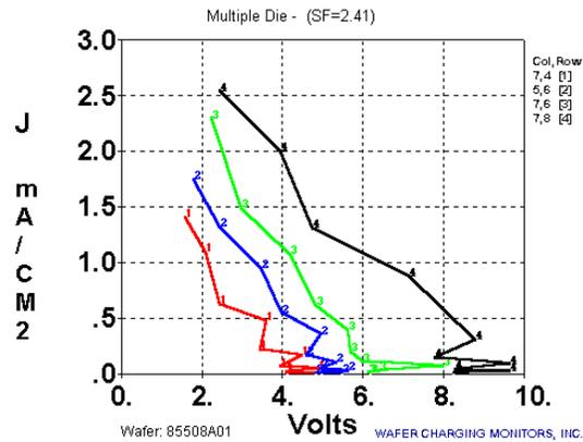
Figure 7. JV plot for Ar plasma exposure case with dc bias case taken for two dies at the center and two dies at the edge of the wafer
