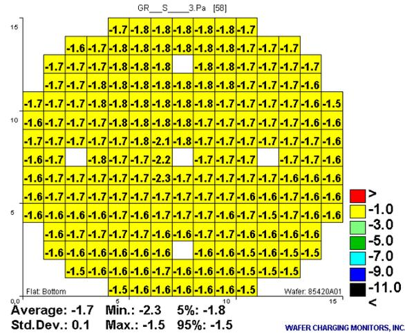
Figure 3. Negative voltage response seen after exposure to Ar plasma with no RF bias
