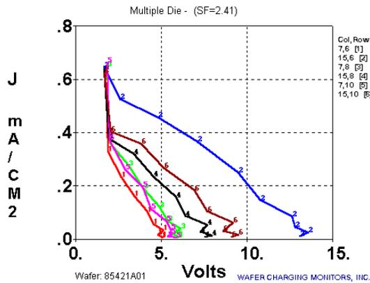
Figure 6. JV plot for  $BCl_3/Cl_2$  etching case taken for two dies at the center and three dies at the edge of the wafer
