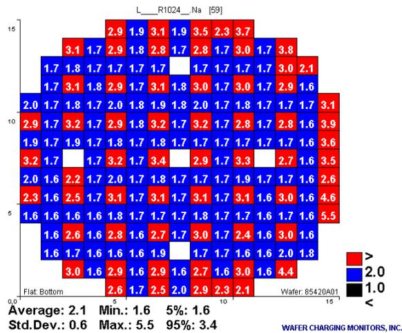
Figure 2. Positive voltage response seen after exposure to Ar plasma with no RF bias
