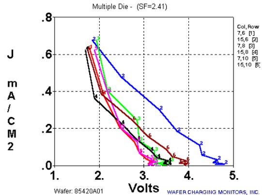
Figure 4. JV plot for Ar plasma exposure case with dc bias case taken for three dies at the center and two dies at the edge of the wafer
