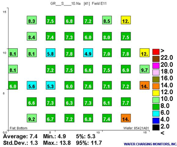
Figure 5. Positive voltage response seen after etching CCE with a  $BCl_3/Cl_2$  discharge
