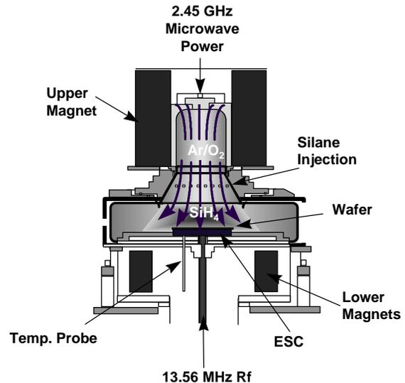
**Fig. 1.** Cross sectional diagram of the ECR-CVD chamber used in this work.
