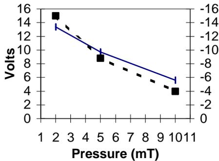
**Fig. 5.** CHARM®-2 maximum peak voltage responses (solid for positive and dashed for negative) after exposure to 30 second high biased depositions as a function of process pressure.
