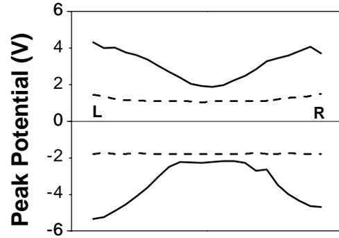
**Fig. 6.** CHARM®-2 Positive and negative voltage responses after exposure to zero bias plasma at 2mT (solid line) and 10mT (dashed line). Note that the wafer used for 10mT case had a lower threshold.
