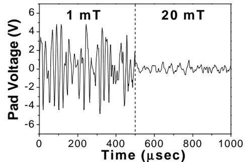
**Fig. 7.** Voltage signals on a SPORT wafer show a frequency of about 30kHz for a zero biased ECR oxygen/argon plasma at 1 and 20 millitorr.
