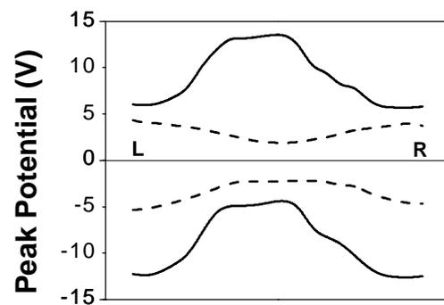
**Fig. 3.** CHARM®-2 Positive and negative voltage response after exposure to zero biased deposition (dashed line) and RF biased deposition (solid line).
