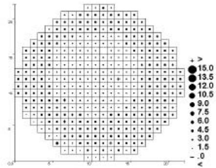
**Fig. 2a.** Positive voltage response after exposure to microwave only (no RF bias) deposition.
