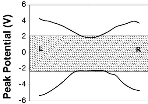
**Fig. 4.** CHARM®-2 Positive and negative voltage response after exposure to zero biased deposition. The hashed region indicates the threshold level.
