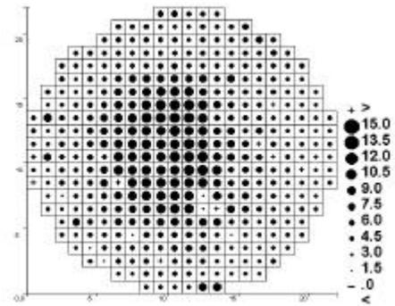
**Fig. 2b.** Positive voltage response after exposure to biased deposition (i.e., a gap fill process).
