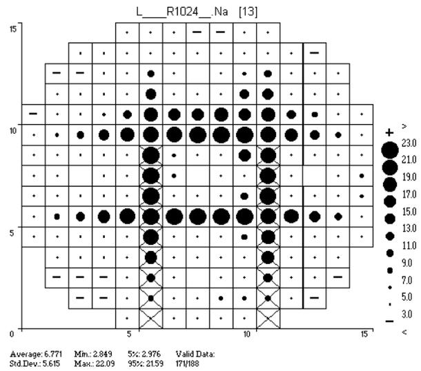
Figure 9. Positive potentials across current sensor on wafer covered with resist patterned with product via mask; "X" indicates die location selected for J-V plot in Figure 10.
