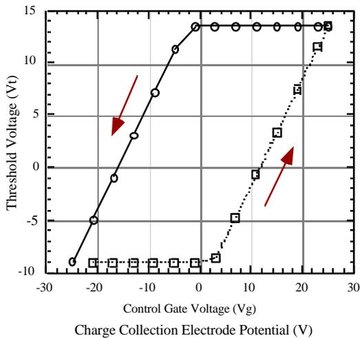
Figure 2. Vg vs. Vt characteristics of CHARM™-2 EEPROM transistor.
