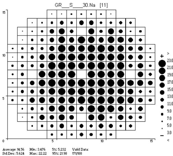
Figure 8. Positive potentials on wafer covered with resist patterned with product via mask.
