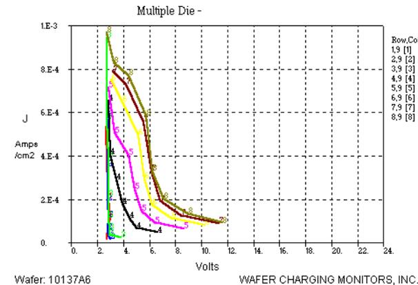
Figure 6. Positive J-V plots obtained on bare wafer.
