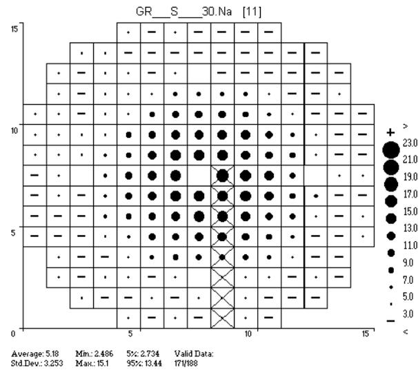
Figure 5. Positive potentials on bare wafer; "X" indicates die location selected for J-V plot in Figure 6.
