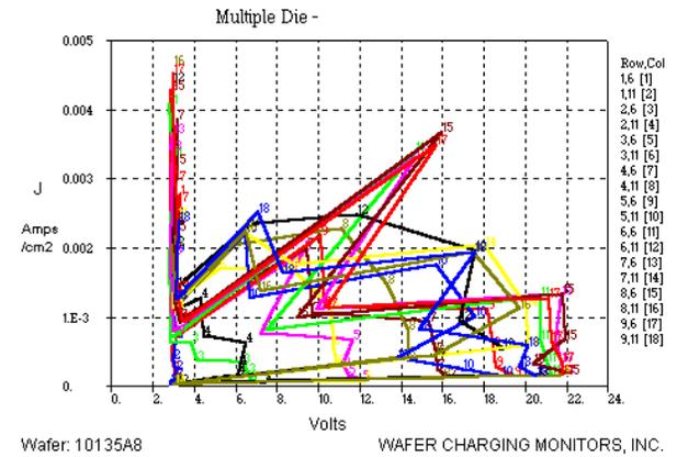
Figure 10. Positive J-V plots obtained on on wafer covered with resist patterned with product via mask. J-V plots are irregular due to mis-alignment of via mask and CHARM™-2 wafer layout. (Note change in J scale. To obtain actual J values, the above results must be multiplied by at least 2.3)
