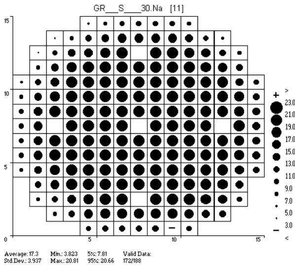
Figure 7. Positive potentials on resist-covered wafer.
