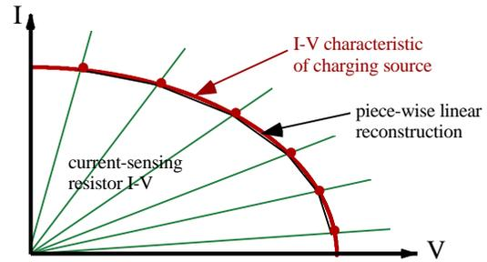
Figure 4. Charge-flux sensors with different value current sensing resistors allow re-construction of the J-V characteristics of the charging source, implementing a passive plasma probe.
