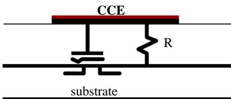
Figure 3. CHARM™-2 charge-flux sensor.
